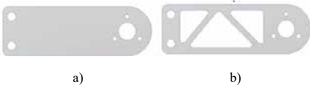
Fig. 18. Optimization of the form of auxiliary link 4 (a – link before optimization, b – link after optimization)
